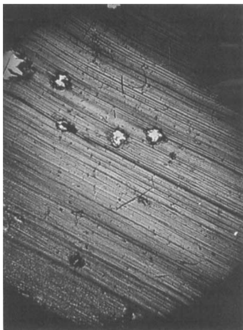
FIGURE 6 Microphotograph of through holes formed in stretched inhibited PP at oxidation under stress; 140°C, air, \sigma = 15 MPa, durability \tau = 198 min. Inhibitor—Irganox 1010.
